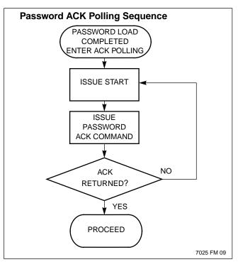
If the password that was inserted was correct, then an "ACK" will be returned once the nonvolatile cycle is over, in response to the ACK polling cycle immediately following it.
