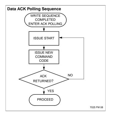
After the password sequence, there is always a nonvolatile write cycle. This is done to discourage random guesses of the password if the device is being tampered with. In order to continue the transaction, the X76F641 requires the master to perform an ACK polling with the specific code of F0h. As with regular Acknowledge polling the user can either time out for 10ms, and then issue the ACK polling once, or continuously loop as described in the flow.
