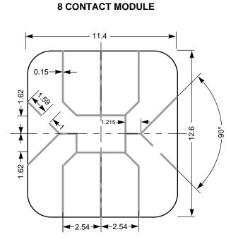
8 PAD CHIP ON BOARD SMART CARD MODULE TYPE X
