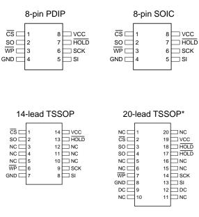
Note: \*Pins 3, 4 and 17, 18 are internally connected for 14-lead TSSOP socket compatibility.
