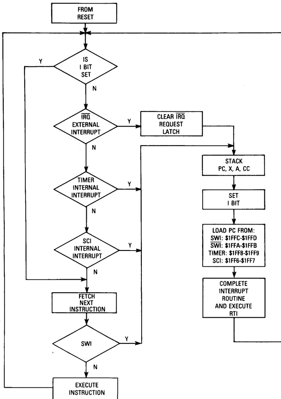
Figure 6. Reset and Interrupt Processing Flowchart
