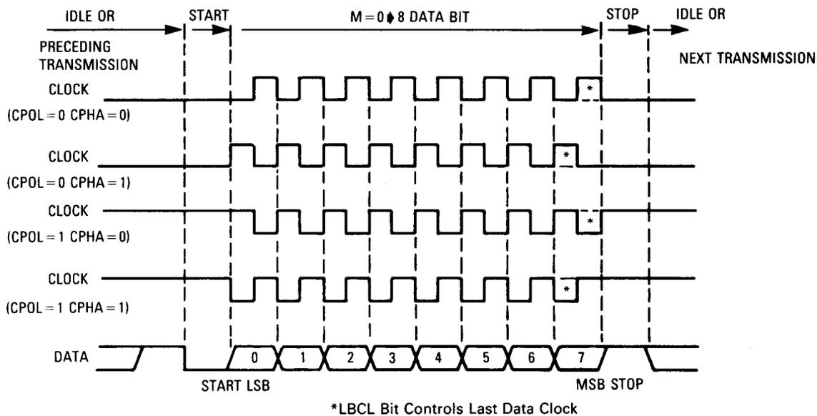
**Figure 13. SCI Data Clock Timing Diagram (M=0)**
