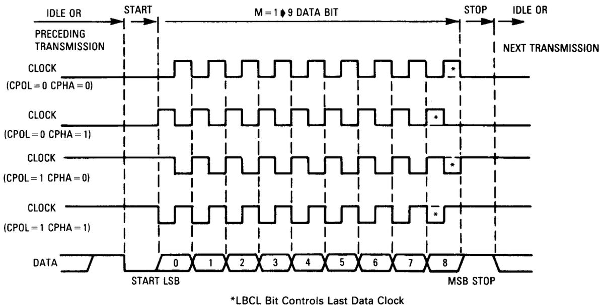
**Figure 14. SCI Data Clock Timing Diagram (M=1)**
