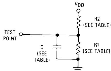
Figure 19. Equivalent Test Load
