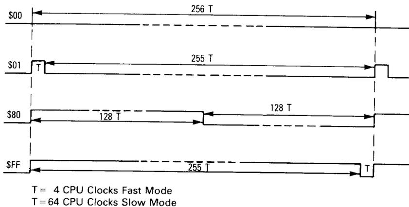
Figure 18. PLM Output Waveform Examples
