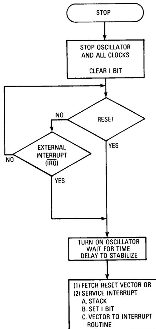
Figure 8. STOP Function Flowchart
