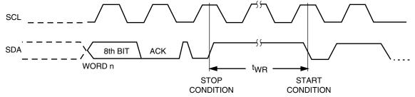
Note: The write cycle time  $(t_{WR})$  is the time from a valid stop condition of a write sequence to the end of the internal erase/program cycle.
