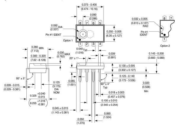
Molded Dual-In-Line Package (N) Package Number N08E
