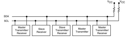
$\textbf{Note:} \qquad \text{Due to open drain configuration of SDA and SCL, a bus-level pull-up resistor is called for, (typical value = <math>4.7 \text{k}\Omega$ )}
